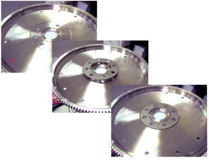
Figure 1: Reuse of the Factory Spacer
